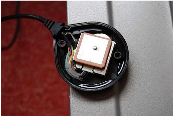
Figure 33: An EM-406A module embedded into the housing of a Fortuna U2, to the left, and embedded into a housing of a Navilock NL-303P, to the right.
