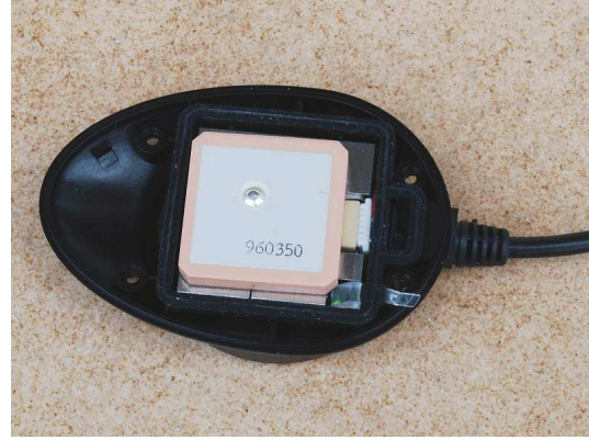
Figure 33: An EM-406A module embedded into the housing of a Fortuna U2, to the left, and embedded into a housing of a Navilock NL-303P, to the right.
