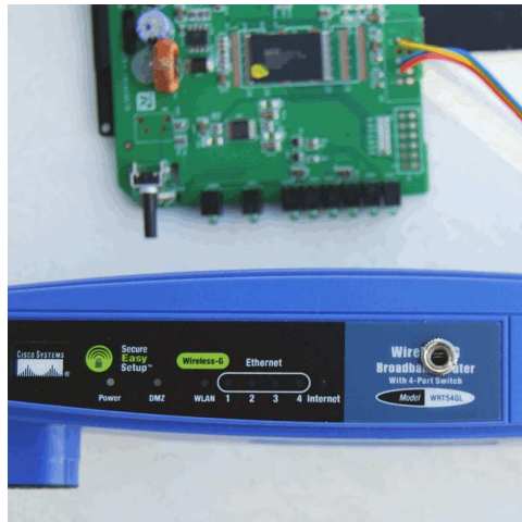
Figure 39: A modified Linksys WRT55GL router.
